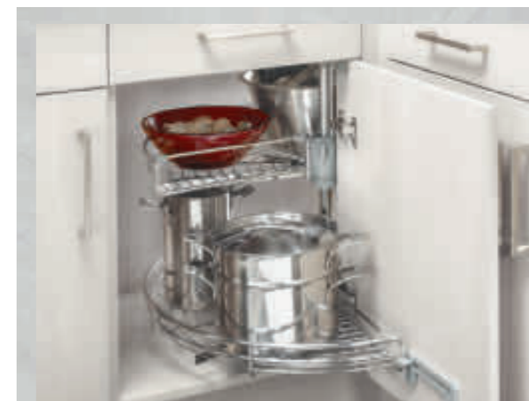
180° Chrome Carousel For Conventional Corner base unit Minimum door width 400mm (800mm base) 450mm (900mm base). Weight capacity - 9kg per shelf 10C180C
